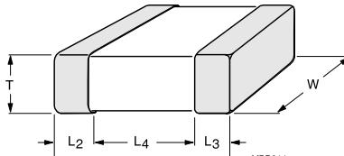
Fig. 2 Surface mounted multilayer ceramic c
